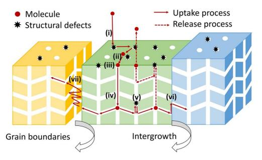
Fig. 1. Illustration of the transport process from the bulk phase into the interior of nanoporous materials. From Xu et al. [5]
